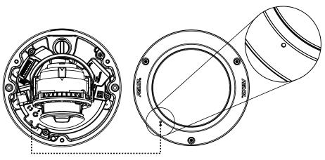
Figure 15. Align Small Hole for Microphone
