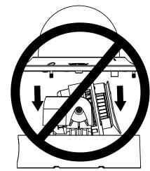
Figure 13. Incorrect Dome Cover Attachment Method
