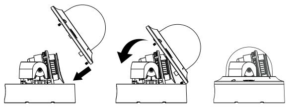
Figure 14. Correct Dome Cover Attachment Method
