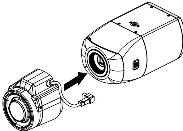
**Figure 3.** Tighten the iCS Lens Onto the Lens Mount
