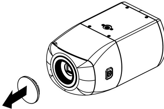
**Figure 2.** Remove the Cover from the Lens Mount
