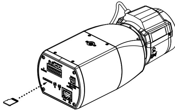
**Figure 5.** Insert a Micro SD Card
