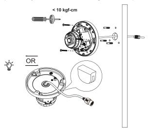
Note: It is always a good practice to form a drip loop on cables. Moisture condensation or dripping water can eventually cause problems without the drip loop.
