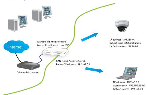
2. If the Local Area Network (LAN) IP address of your Network Camera is 192.168.0.3, forward the following ports for the Network Camera on the router.
