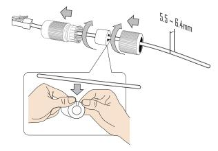
7. Install the seal ring and tighten the waterproof components.
