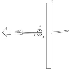
6. Pass an Ethernet cable through the waterproof cable gland components, and through the rubber seal as shown below. Connect the Ethernet cable to the camera's RJ45 connector.
