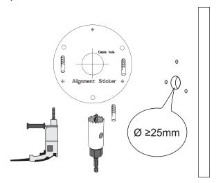
4. Route an Ethernet cable through the cabling hole.
