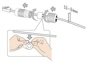
6. Install the seal ring and tighten the waterproof components.
