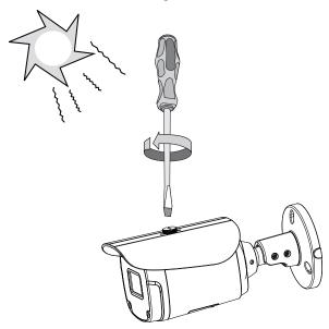
9. Install the camera to wall using the included screws. Note that if a routing hole through the wall is not possible, you can also route the cable through the side opening.
