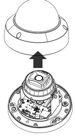
Make sure the rubber seal is properly installed to the center hole. The outer rim of the seal must be through and cover the
