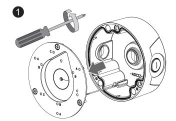
A 3/4" conduit is required for routing the cables with waterproof
