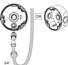
Attach the included alignment sticker to a preferred position. Drill holes on the wall and install the junction box. If space behind the wall allows, you may also pass cables through the wall.
