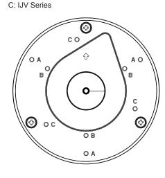
Pass the camera's Ethernet cable through the center hole of the box and the rubber seal.
